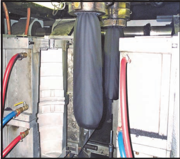
Parison dropping down into open mold before forming
